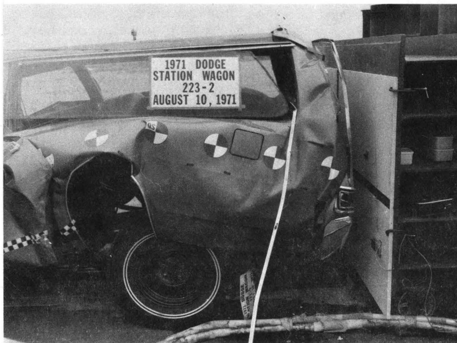
Figure 5-31. Dodge Station Wagon Impact Damage From 27.6-mph Barrier Test.
