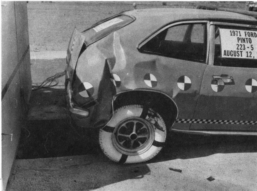
Figure 5-30. Pinto Impact Damage From 20.1-mph Barrier Test.
