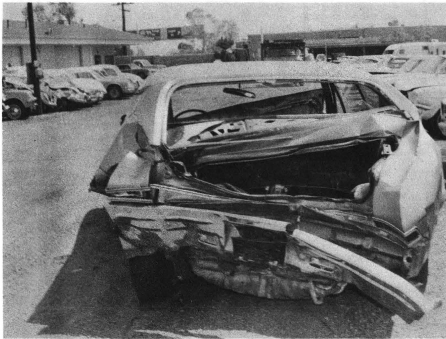
Figure 5-44. Severe Rear End Collision Damage in 1971 Chevelle Malibu.
