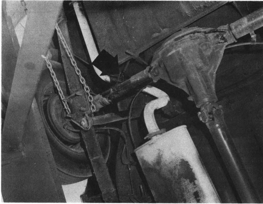
Figure 5-57. Fuel Spillage From Damaged Vapor Hose in AMC Hornet.
