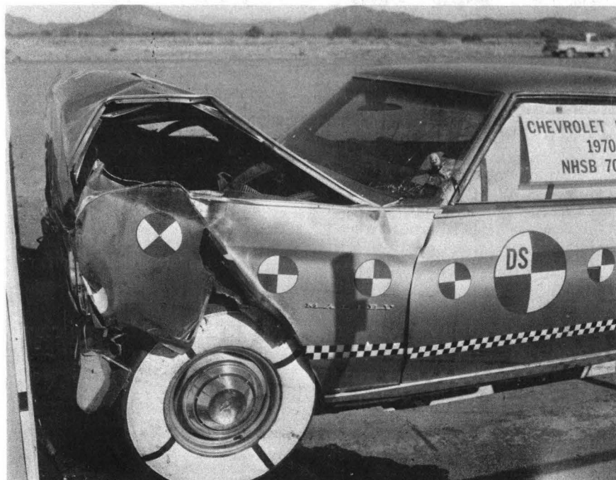
Figure 5-18. 1970 Chevelle Malibu After 30-mph Barrier Test.
