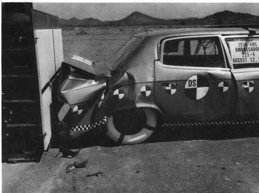
Figure 5-29. Ambassador Impact Damage From 20.2-mph Barrier Test.
