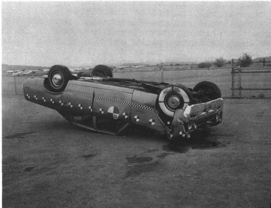
Figure 5-59. Inverted Resting Position of AMC Ambassador.
