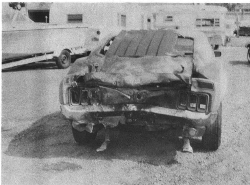
Figure 5-51. Fire Damage in 1970 Mustang Involved in Moderate Rear End Collision.
