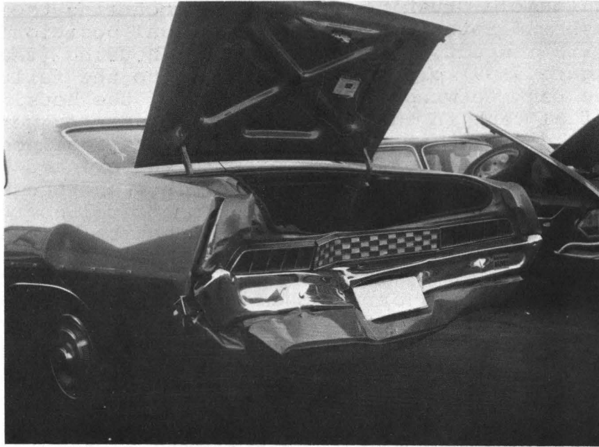
Figure 5-42. Rear End Collision Damage to 1970 Ford Torino.
