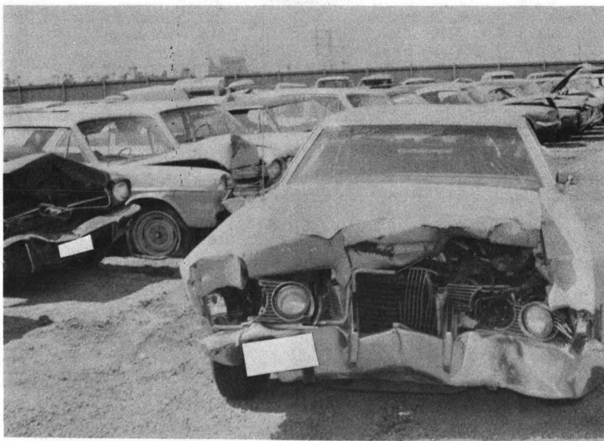
Figure 5-21. 1971 Cougar Involved in a Moderate Front End Collision.
