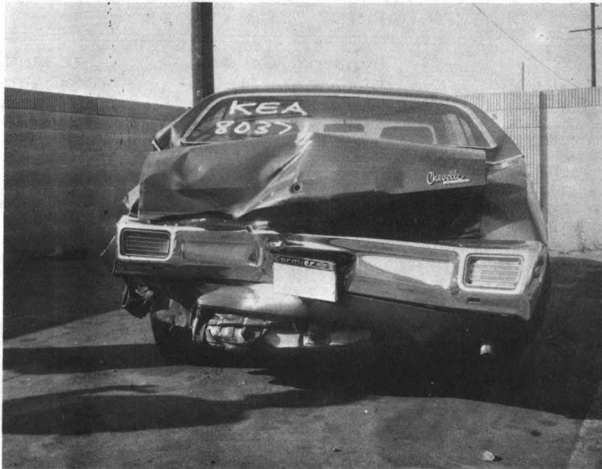
Figure 5-40. Rear End Collision Damage to 1970 Chevelle.
