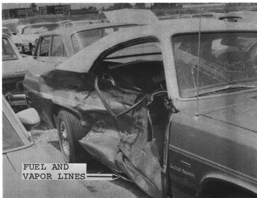
Figure 5-53. Typical Side Impact Damage.
