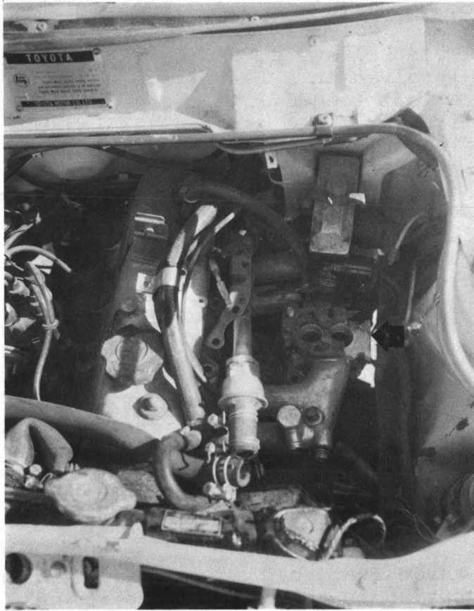
Figure 5-19. Broken Carburetor Mounting in Barrier-Crashed Toyota Corolla.
