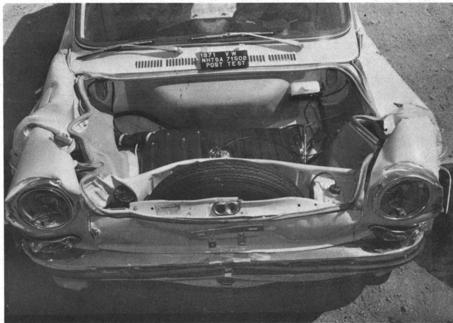
Figure 5-14. 1971 Volkswagen Squareback After a 30-mph Barrier Impact.
