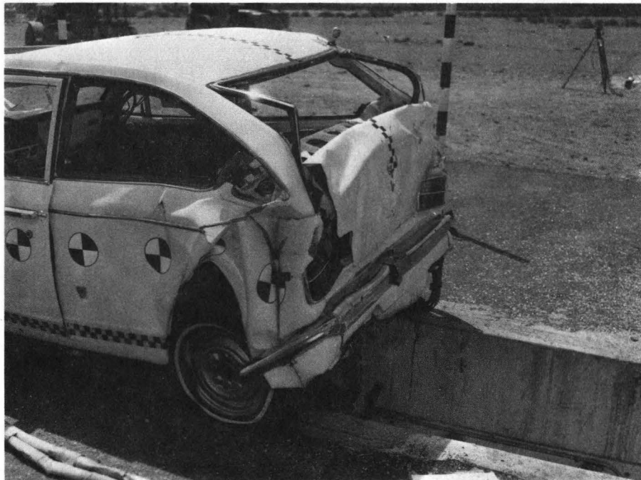
Figure 5-27. Toyota Impact Damage From 30.2-mph Barrier Test.
