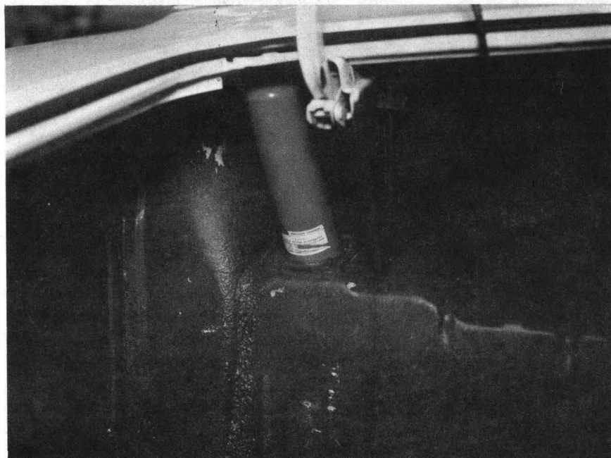
Figure 4-2. 1970 Ford Galaxie Liquid-Vapor Separator.
